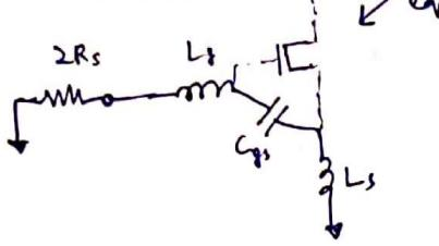
↳ equivalent circuit at resonance
